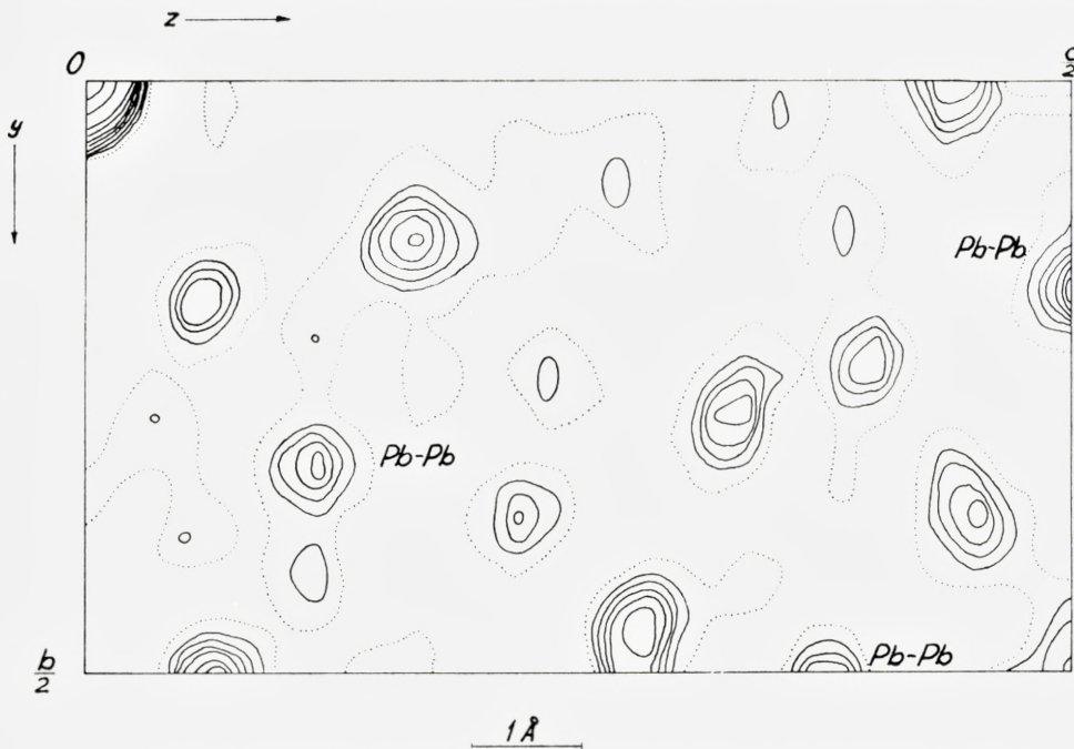
Fig. 1. Patterson projection of yellow CsPbI_3 on the bc -plane. Contour lines are drawn at the relative densities 0, 40, 60, 80, 100, 125, 150, 200, 600, 800.
